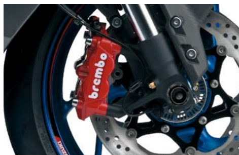
Colour Brembo calipers 59100-17800-000 OE replacement / Red. (W/O Pads)
